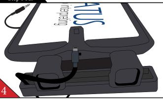
Lift the tab of the case and attach the power lightning USB cable from the stand into the side of the iPad. If the stand has the speaker option attachment, the audio speaker cable on the lower end of other side.
