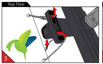
Tilt the top of the head down to attach the Stratus Flipcover instruction guide using the two ball chains provided. Assure the logo side is placed on the front while assessing the instruction side when flipped.
