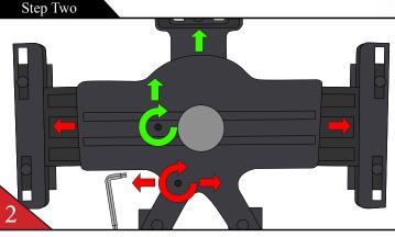
Insert the key firmly into the keyhole to unlock the iPad placement mounts. The lower keyhole unlocks the sides, while the upper one unlocks the top one. Firmly pull apart arms after turning the key in a clockwise manner.
