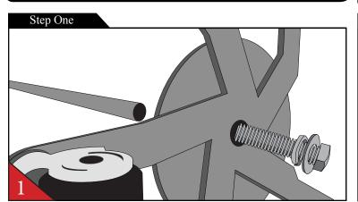
Lay the Base Assembly on its side while vertically aligning the Pole Assembly through the center. Connect together the Bolt and Washers using the Wrench turning clockwise to tighten.
